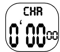
Press SET/LIGHT/STP/RST. to reset the stopwatch, then press ADV./ST./SPL. to start it.
